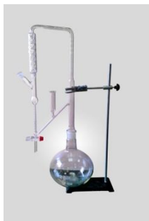
Fig S1. Extraction by Hydrodistillation
