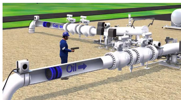
Figure 4. Difference between pig locating and pig tracking [4]
