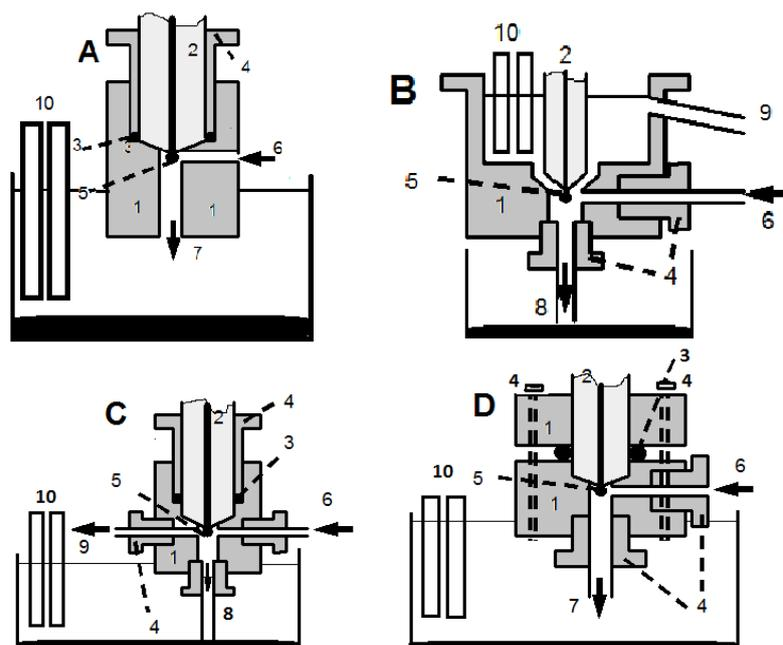
**Fig. 1.** View of four tested flow-through cells. (1) PMMA Cell body, (2) glass capillary of the SMDE, (3) o-ring, (4) fixation screw, (5) mercury drop, (6) solution inlet, (7) solution and mercury outlet, (8) mercury outlet, (9) solution outlet, and (10) auxiliary and reference electrode
