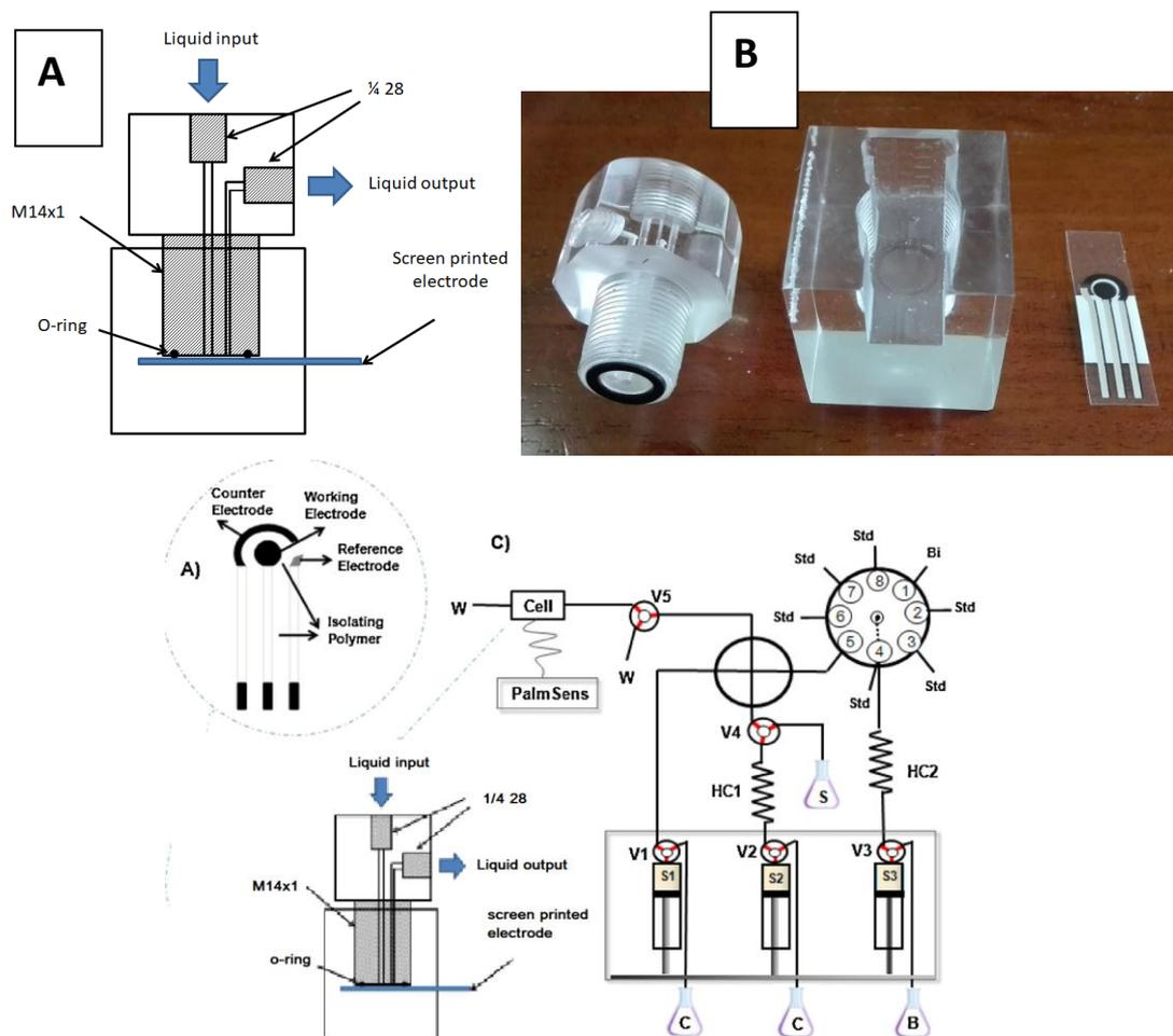
**Fig. 3.** A) Schematic representation of the flow cell and B) Photo of home-made components of the flow cell, including the screen printed electrode.
