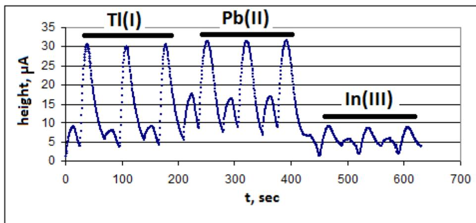
**Fig. 6.** Consecutive amperometric detection of Tl(I), Pb(II), and In(III). Sample size 70 µL, electrode area 1.02 mm<sup>2</sup>. Ions concentrations: Tl(I) 6.4x10<sup>-3</sup> mol L<sup>-1</sup>, Pb(II), and In(III) 8x10<sup>-3</sup> mol L<sup>-1</sup>. DPV mode.
