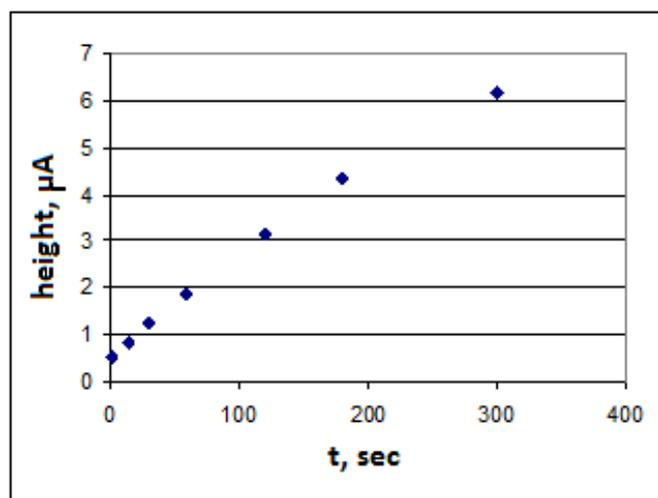
**Fig. 7.** Variation of the analytical signal with accumulation time for  $6 \times 10^{-6}$  mol L<sup>-1</sup> Cd in 0.01 mol L<sup>-1</sup> HCl. Electrode area 1.16 mm<sup>2</sup>. DPV mode. Accumulation potential -700 mV, pulse amplitude 50 mV, scanning speed 25 mV s<sup>-1</sup>, pulses duration 100 ms.
