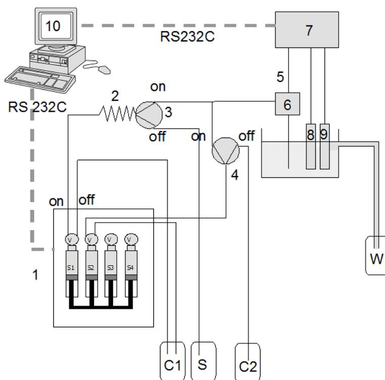
**Fig. 2.** Diagram of the manifold. (1) multisyringe burette, (2) holding coil, (3) and (4) three-way solenoid valves, (5) SMDE, (6) flow-through cell, (7) potentiostat, (8) reference electrode, (9) auxiliary electrode, and (10) personal computer, (W) waste, (S) sample, (C1) Carrier, and (C2) Carrier or NaOH ; (- - -) RS232C connections; S1, S2, S3, and S4 syringes; V three-way solenoid valve
