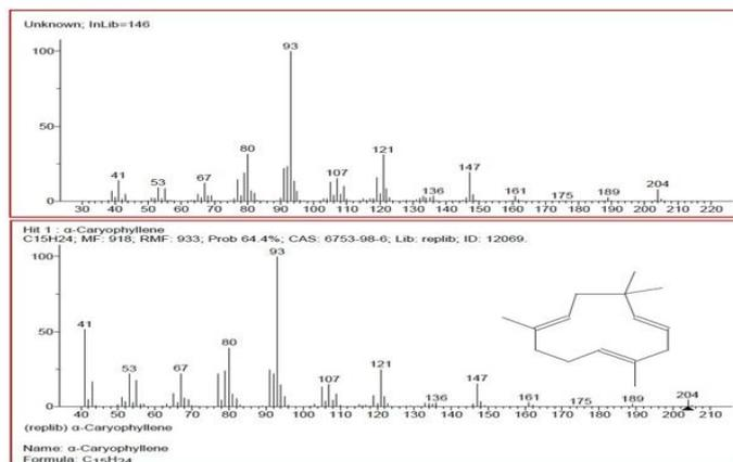
**Fig 2.** The mass spectrum obtained from the GC/MS device and the standard  $\alpha$ -Caryophyllene spectrum after extraction from the upper space
